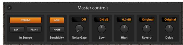
The **In Source** area is where you select the input channels for TH3. You can take a stereo couple as input, or only one of the stereo channels: **Left** or **Right**.
