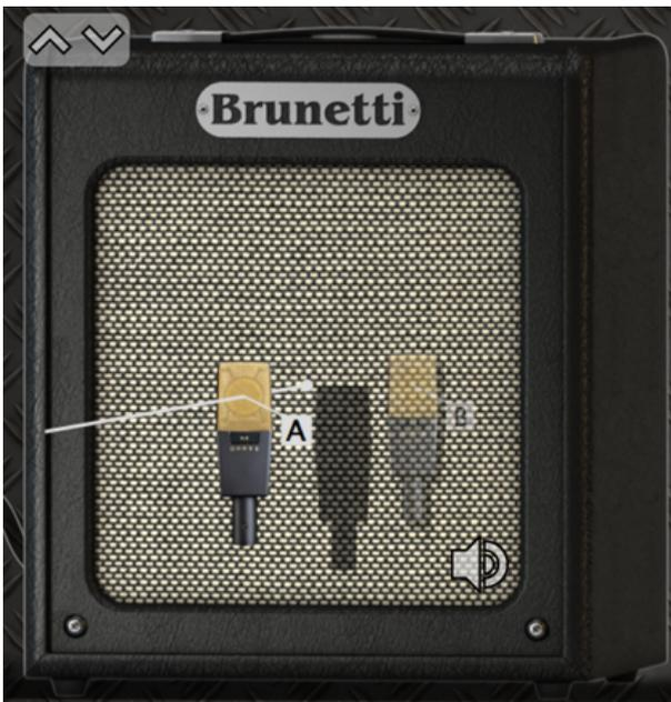
When you right drag the microphone, a white line shows you the Z axis and the microphone shadow projected over the cabinet helps you to make a clearer idea about the distance.
