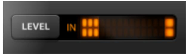
You should try to keep the input level as high as possible without reaching the saturation. You can get assisted to set the correct IN level by clicking the **LEVEL** button as described above.
