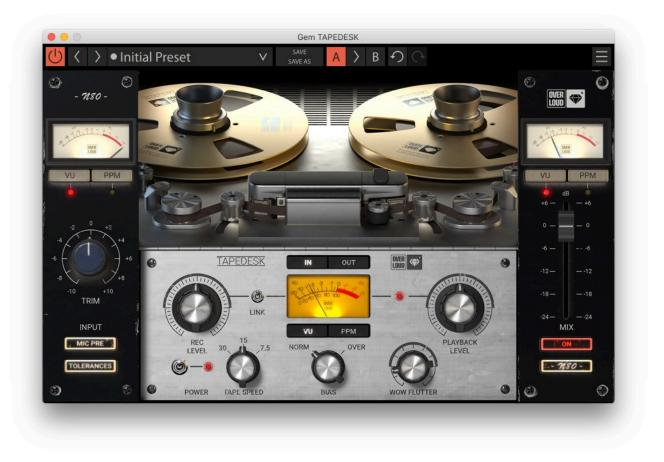
**VU METERS** - **TAPEDESK** has three Meters: two from the mixer and one in the tape machine. All three can be switched between VU or PPM modes.
