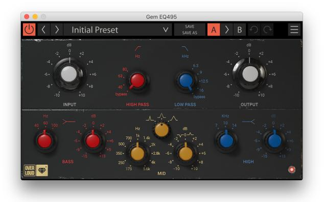
**INPUT** - Adjusts the level of the input signal.
