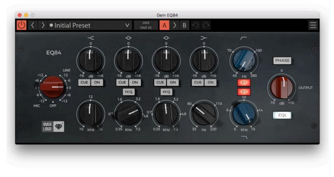
The graphic interface includes the red input gain knob on the left, then four vertical pairs of black knobs and buttons to control frequencies and bands, and then two blue knobs for high and low pass filters. Finally two more buttons on the right side to switch the EQ section on/off and invert the signal phase.
