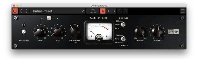
**OVERDRIVE** - Adds 20dB of extra gain to the distortion valve. When switched off the processor produces a gentle saturation: if switched on, highly distorted tones can be obtained.
