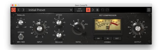
**PARALLEL** - Sets the balance between DRY and COMP (processed) sounds. This is commonly called Parallel Compression.
