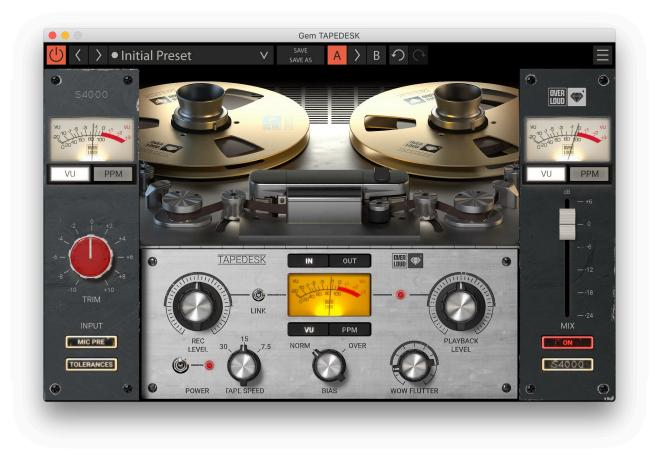
The graphic interface has three areas: the console input channel on the left side, the tape simulator in the middle, and the console mix bus on the right side. The signal path begins at the input
