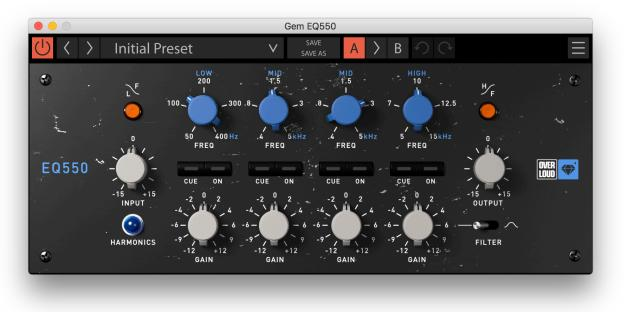
**INPUT GAIN** - This knob controls the input gain. It ranges from -15 dB to +15 dB.
