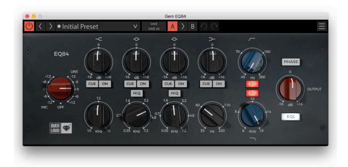
The graphic interface includes the red input gain knob on the left, then four vertical pairs of black knobs and buttons to control frequencies and bands, and then two blue knobs for high and low pass filters. Finally two more buttons on the right side to switch the EQ section on/off and invert the signal phase.
