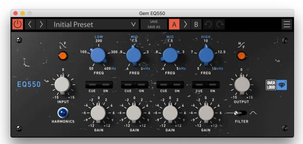
INPUT GAIN - This knob controls the input gain. It ranges from -15 dB to +15 dB.
