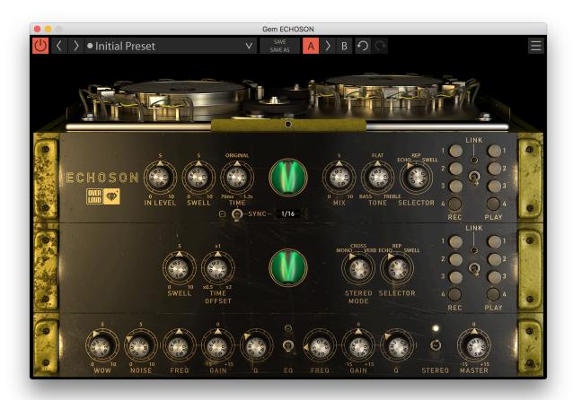
As done for other Gems, this model goes beyond the original modeled unit features. Some of the differences can be found in the added parameters (see descriptions), but the main difference is the option to double the processor panel to have it working on a stereo pair of audio channels.
