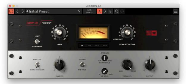
First model (2A) had the electro-luminescent light powered by a tube, while the next one (3A) used a transistor. Tubes can provide less current than transistors, so their response to attack transients was softer and had more harmonics due to the slight distortion introduced.
