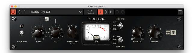
**OVERDRIVE** - Adds 20dB of extra gain to the distortion valve. When switched off the processor produces a gentle saturation: if switched on, highly distorted tones can be obtained.
