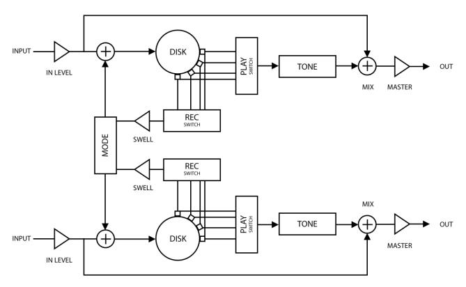
This diagram describes the **ECHOSON** internal sections and the way they are interconnected.
